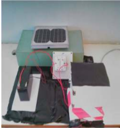
Fig:F Photograph of solar water cooler
