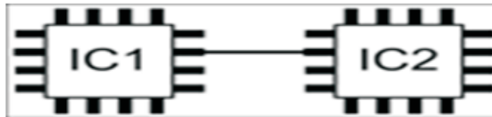
Figure 1. A simple connection is a direct connection from one IC to another.
