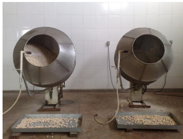
Figure 8 - toasters or drajadeiras during the process to assist carmelization and toasting. Source: photo taken by the authors. (2009)
