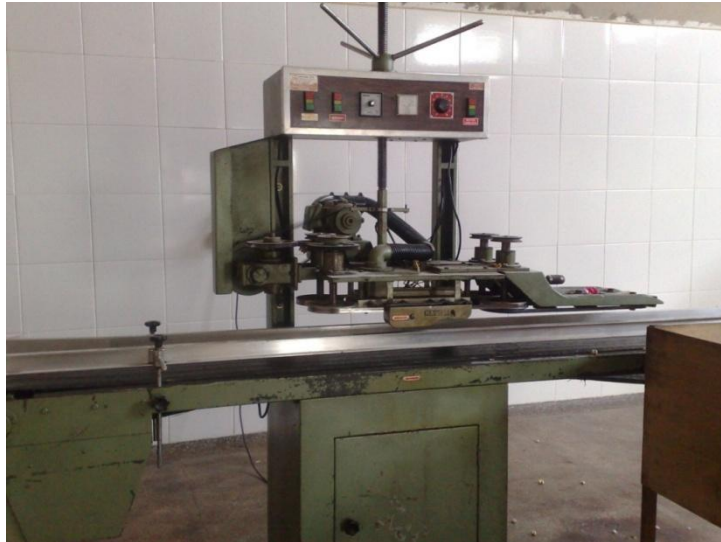
Figure 9 - Sealing of track used for closing bags of red. Source: photo taken by the authors. (2009)
